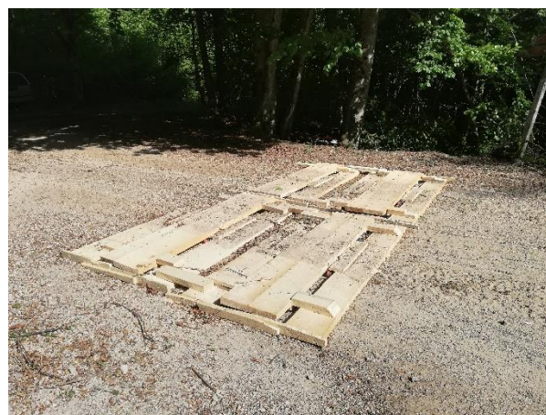
Figure 4: Wooden protection for weighing scales.
