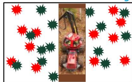
Figure 2: Comparison of boom corridor and selective thinning techniques (photo: Christian Höök)
