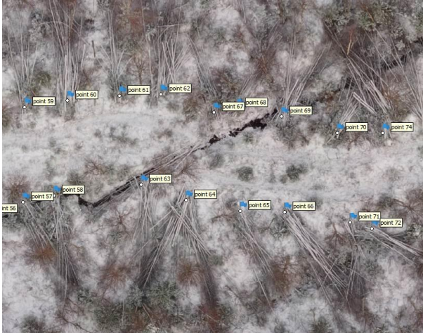
Picture 4. Orthophoto generated from UAV photography showing part of a strip road post harvesting in Finland. Points were manually placed on bunches of trees for quantification of bunch variation between treatments in the study.
